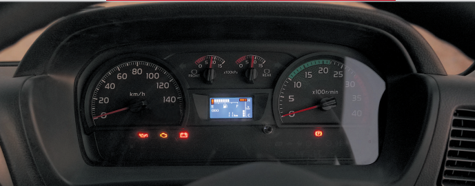
Driver's Instrument Panel New Hino 500 Series is equipped with an instrument panel, which is designed to be read from various angles and in varying lighting conditions, every model is equipped with tachometer, speedometer and a full suite of warning gauges and lights.
