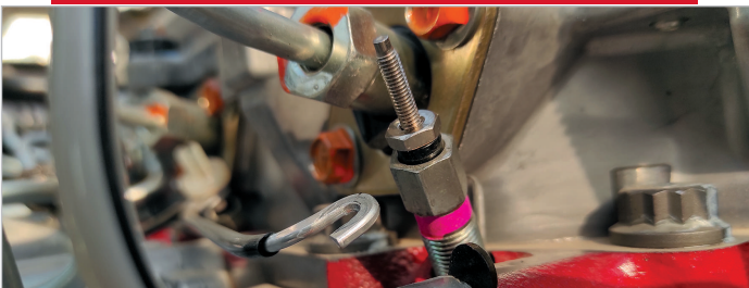
Engine Cold Start System Now be in command in extreme cold weather conditions with the new engine cold start system in the New Hino 500 Series that uses the air pre-heat system to assist in starting the engine when the temperature is below zero degree centigrade.
