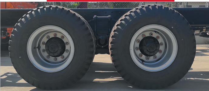
Hub Bolt Type The New Hino 500 Series is now equipped with ISO 10-stud type bolts which reduces weight transfer ratio on each bolt.
