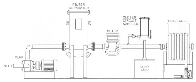
Fuel enters the sampler tangentially at the bottom, creating a clockwise swirl to force particles and water to the center of the coned-down, white epoxy chamber bottom. Any contaminants are then easily seen. After inspection or testing, simply open the outlet valve to release the contents to the dump or slop tank.but the range has been reduced so they will fit in the Aljac sampler.
